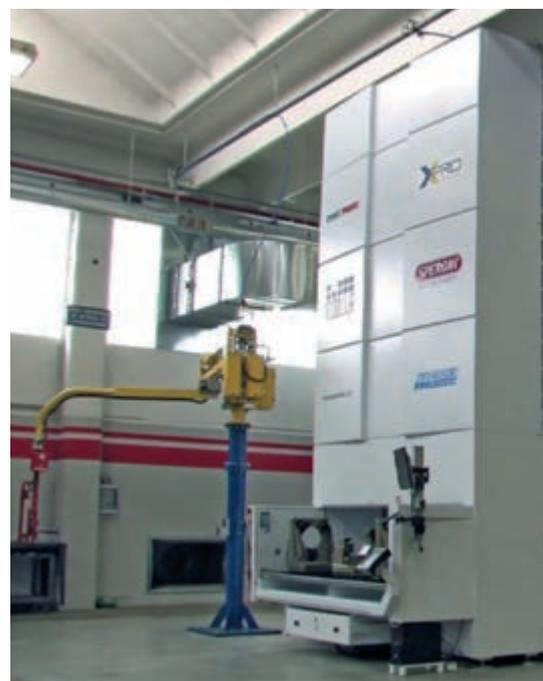
**The SPERONI S.p.A. products they are born from accurate design and strict technical tests.** The test room submits each prototype to a long series of tests to verify the validity of the innovative solutions designed during the design phase. Endurance tests for hundreds of hours of continuous operation in extreme conditions provide invaluable indications for finalizing the final version of the prototype that will move on to the next phase of industrialization.
